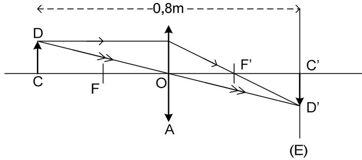
On a  $\overline{CD} = -\overline{CD'}$  or  $\frac{\overline{CD}}{\overline{CD'}} = \frac{\overline{OC}}{\overline{OC'}} \Rightarrow \overline{OC} = -\overline{OC'}$ , de plus
